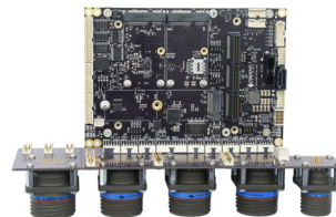
GEODE rugged computer system Internal construction features cable-eliminating I/O board (left) and conduction cooled COM-based CPU (right)
