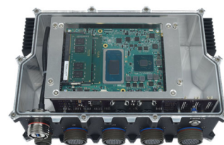
GEODE rugged computer system Internal construction features cable-eliminating I/O board (left) and conduction cooled COM-based CPU (right)
