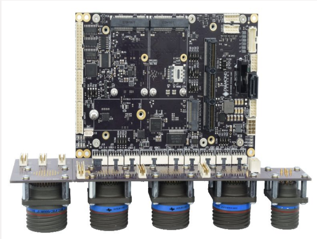
Internal construction showing B2B connection between Jasper COM carrier and connector board
